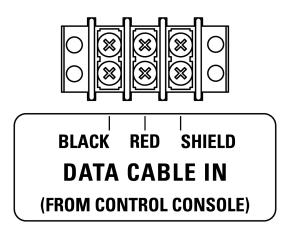
You may purchase data cable from Electro-Mech, or you may source it elsewhere. We recommend (and supply) cable that is rated for direct burial. It includes two insulated 22 AWG stranded conductors (red and black), along with a non-insulated conductor, all wrapped by a braided or foil shield. This document will discuss, in a few pages, what the other end of this cable is connected to.
